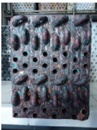
Cu/Cu heat exchanger without coating – Inspection after 1000 hours: the fin surface and the tubes appear completely oxidized
