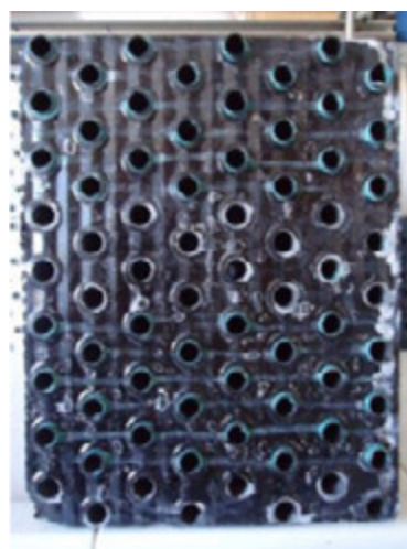
Cu/Al heat exchanger with ELECTROFIN coating – Inspection after 3500 hours: no attack is visible
